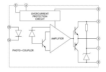
Figure 1. IGBT Driver, Pin Description and Schematic
