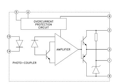
Figure 5-3 IGBT Driver, Pin Description and Schematic
