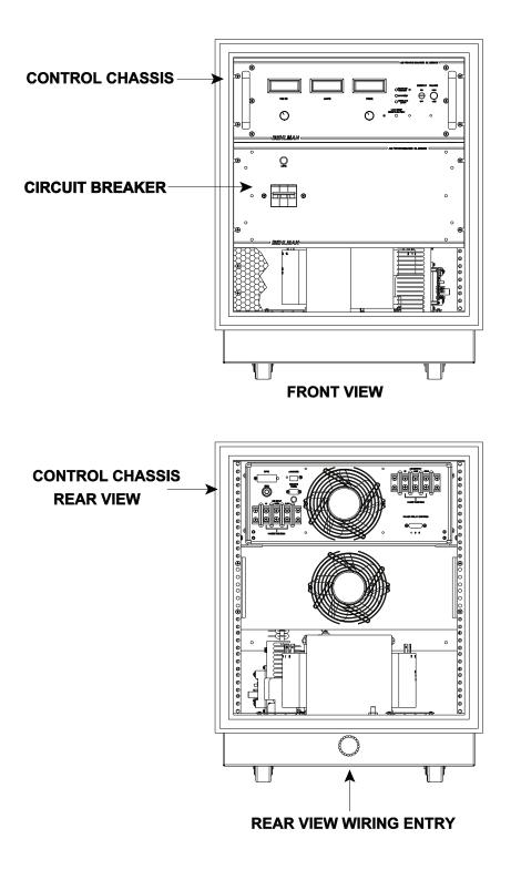
Figure 3-2 Typical BL 20000 Front and Rear Panel Views
